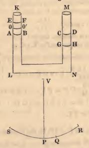
altitude of the water in the two arms of the vessel to be A B, C D. Then when the water in the arm K L has ascended to E F, the water in the arm M N will descend to G H, and the moving force of the water equals the excess of the water in one arm above the water in the other, equals twice A E F B. Let V P be a pendulum, R S a cycloid =  $\frac{1}{2}$  length of the canal, and P Q = A E. The accelerating force of the water : whole weight :: A E or P Q : P R.
